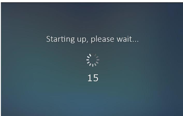
2. During startup, the system is sequentially turning on AV equipment, initializing volume levels, and setting video routes. A countdown timer is displayed to indicate the progress of the startup sequence.
