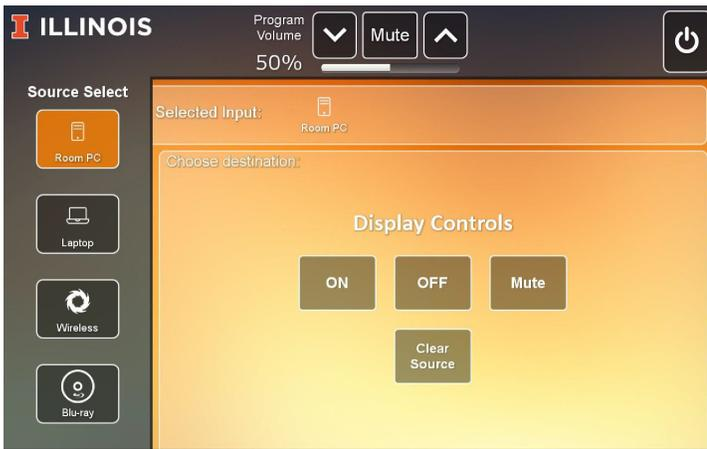
4. Press the desired source button in the “Source Select” pane to select a video source to send to all displays. The selected source will be highlighted. Contextual information about the source will be displayed on the right.
