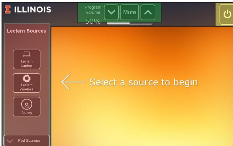
3. Choose a video/audio source to route to a destination. (See “Main: Source Selection” for detailed information on routing controls). Sources are displayed in two separate groups: “Lectern Sources” for sources associated with the instructor location and “Pod Sources” for the individual group input locations around the room.
